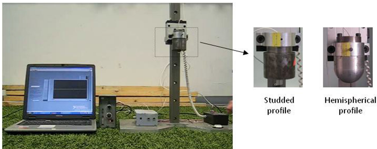
Fig. 1 SERG drop hammer setup and studded hammer profile and hemispherical hammer profile, modified from Carré et al. [25]. (Note: the studded profile presented here is not that used for testing—see Table 1)
