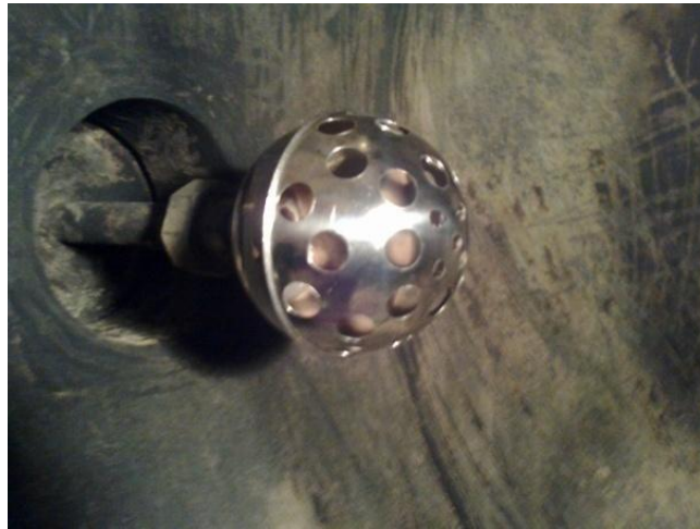
Figure 2. The spherical grid dust disperser.
