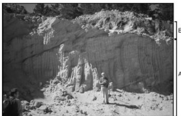
Fig. 3. Exposure of lower aeolianite unit at in the Wilderness seaward cordon with (A) calcified sand with high-angle bedding, (B) iron staining of upper surface associated with inferred palaeosol.
