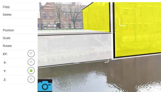
Fig. 4: Real-time construction of occlusion geometry. Cuboids may be translated, scaled, and rotated about a selected axis.
