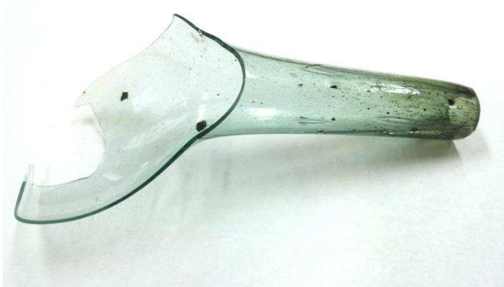
Fig. 4: Iron oxide scale from a blowing iron dissolving in a Roman-type glass during an experimental glassworking project by Mark Hill and David Taylor; the affected glass turns green demonstrating how contamination can alter the glass colour.
