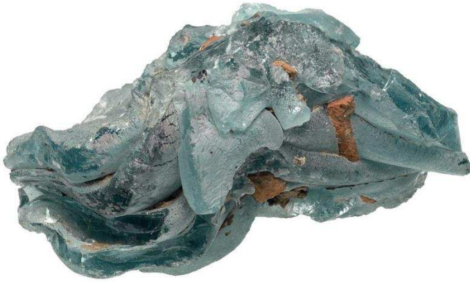
Fig. 8. Partially melted Roman windows amongst a cullet dump from Basinghall, London (courtesy of MOLA). The adhering material would result in contamination of the glass.
