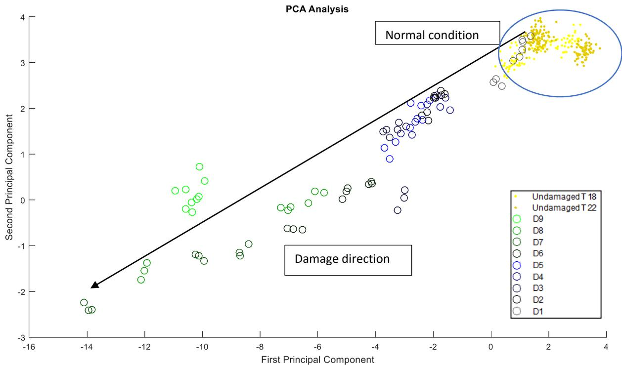
Figure 6: First two principal component scores of the AR parameters related to damage scenarios
