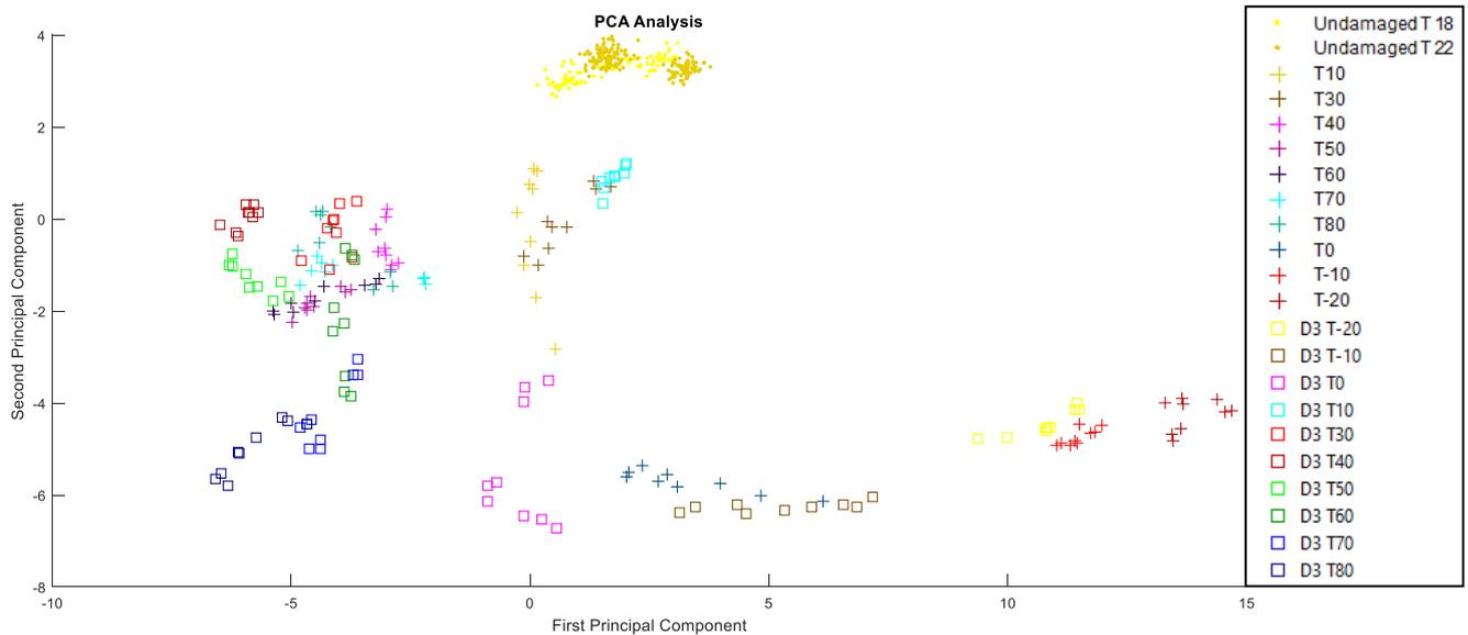
Figure 10: First two principal component of the AR parameters related to temperature variations and 3<sup>rd</sup> level of damage plus temperature variations
