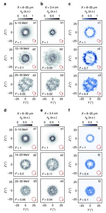
Figure 3 | 3D-PIC simulations results showing the proton spatial-density distribution for elliptical and circular polarization. (a-c) Same caption as Fig. 2d-f, for elliptically polarized light. (d-f) Same for circularly polarized light.
