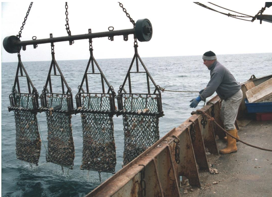
Figure 1.3. A gang of spring toothed, Newhaven scallop dredges during retrieval ( Photo: B. Beukers-Stewart )
