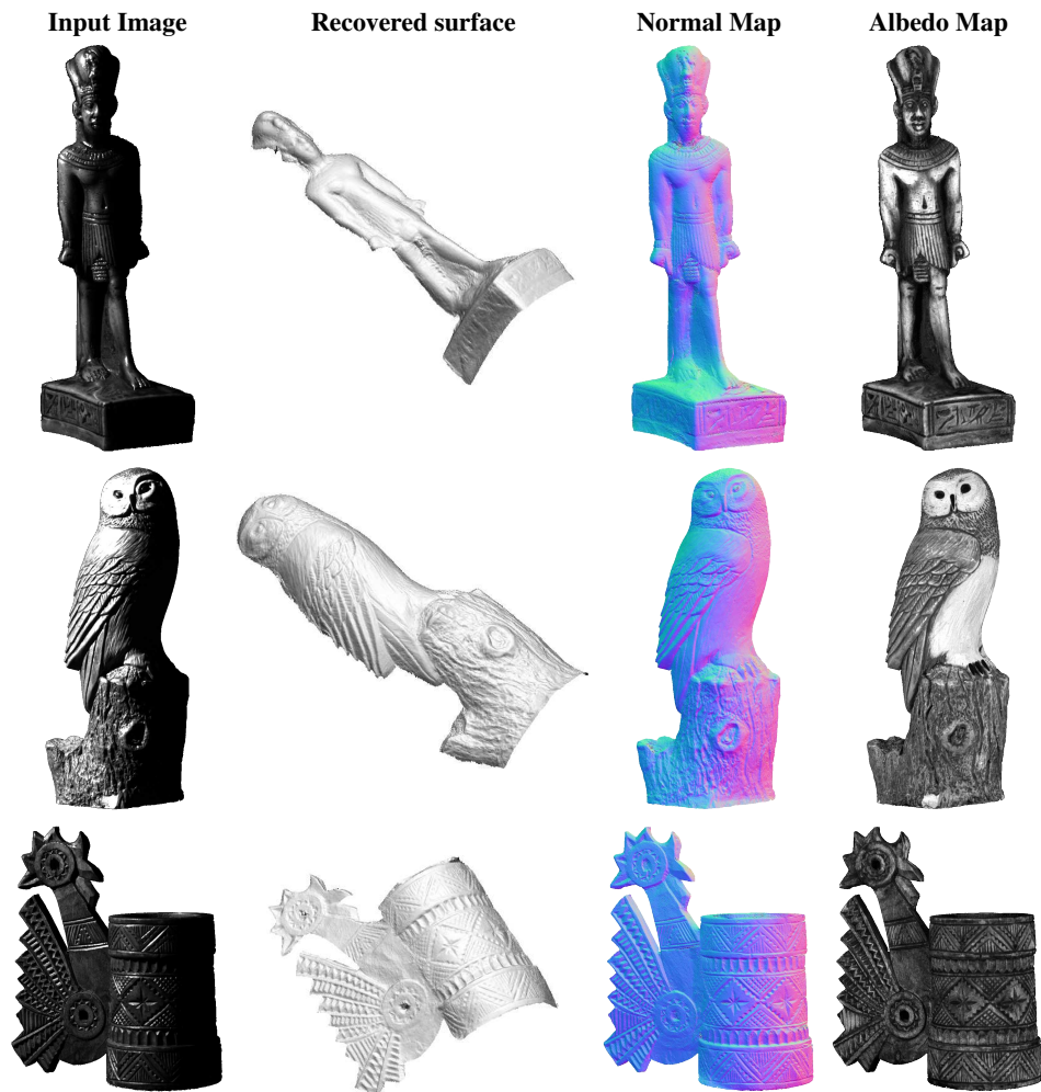
Figure 7: Qualitative results for our own data collected in a lightstage. Input images (col. 1) contain both cast shadows and strong specular reflections. Col. 2 shows reconstructed surfaces in a novel view. Col. 3 shows the surface normals of the reconstructed surface and col. 4 the albedo map.
