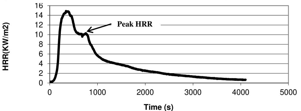
Figure 5. HRR by oxygen mass consumption v. time
