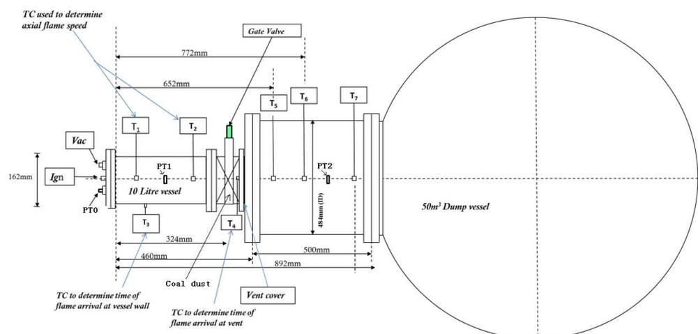
Figure 2: Experimental set-up for vented explosions.
