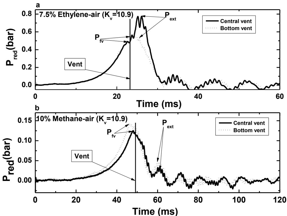
Figure 3: Pressure-time records of central and bottom vent positions for  $K_v=10.9$ .
