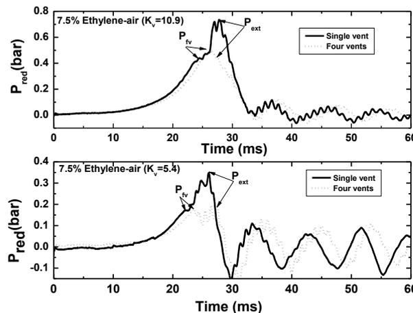
Fig. 6: Pressure-time records for single and four vents for 7.5% Ethylene-air  $K_v=10.9$  and 5.4.
