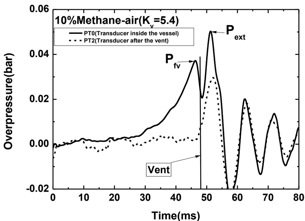
Figure 1: Pressure-time records of PT0 and PT2 for 10% methane-air.
