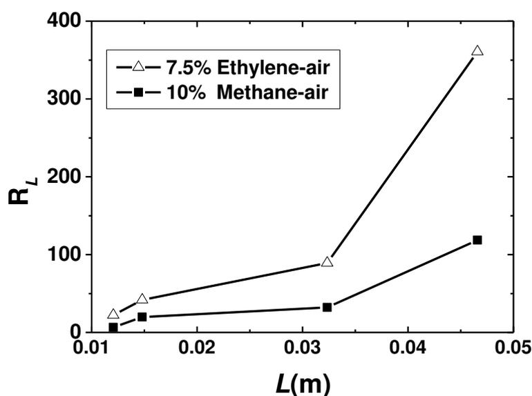
Figure 8: Obstacle length scale as a function of  $R_L$  for 10% methane-air and 7.5% ethylene-air.
