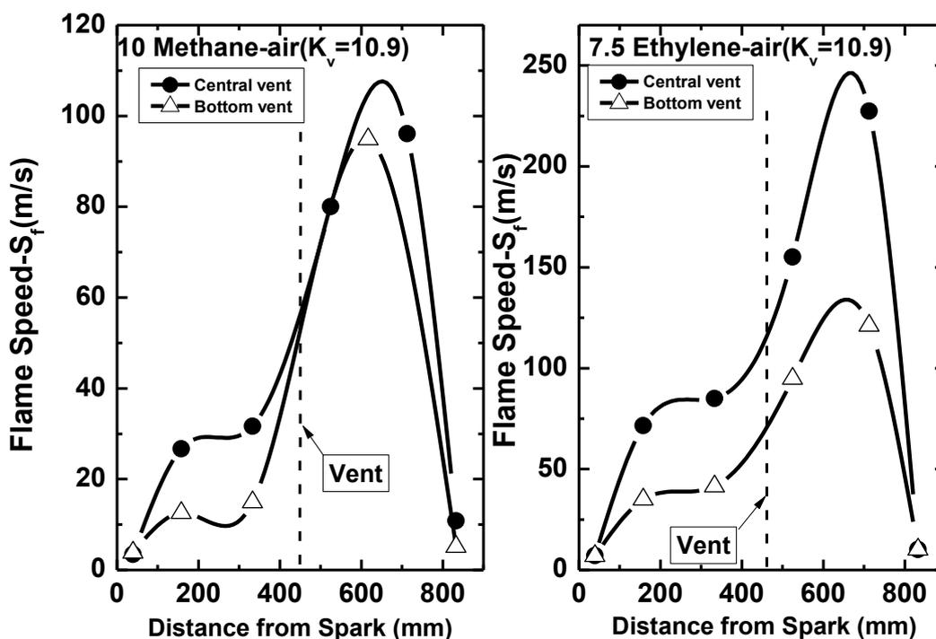
Figure 4: Flame speed vs distance from spark of central and bottom vent positions for  $K_v=10.9$ .
