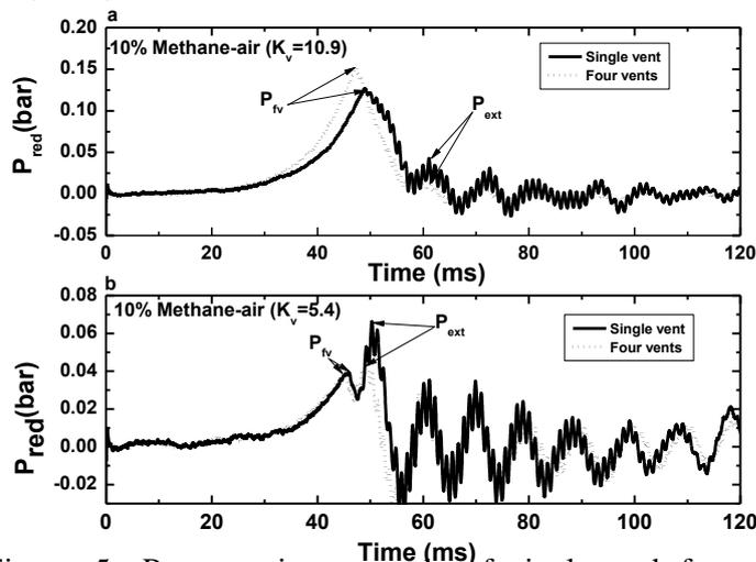
Figure 5: Pressure-time records of single and four vents for 10% Methane-air  $K_v=10.9$  and 5.4.
