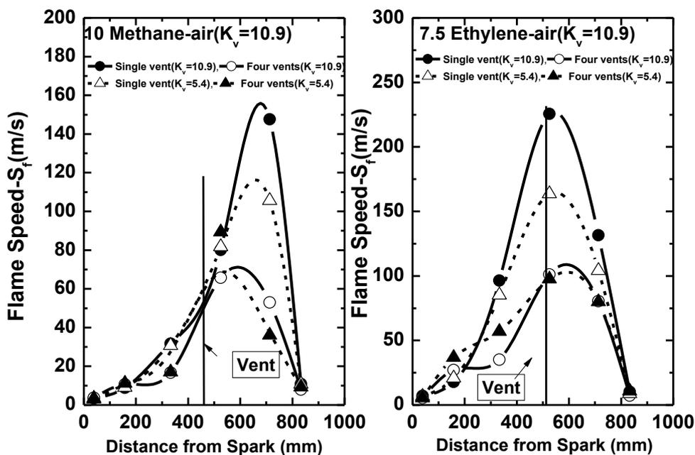
Figure 7: Flame speed vs distance from spark of single and four vents for  $K_v=10.9$  and 5.4.
