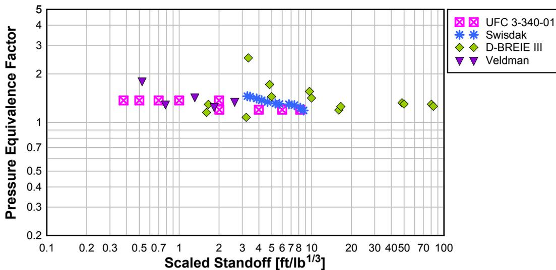
Figure 1: Pressure equivalence data for C-4 in STREET.
