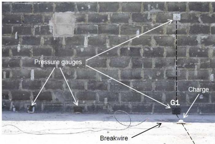
Figure 7: Typical experimental setup for PE4 tests (from [13]).
