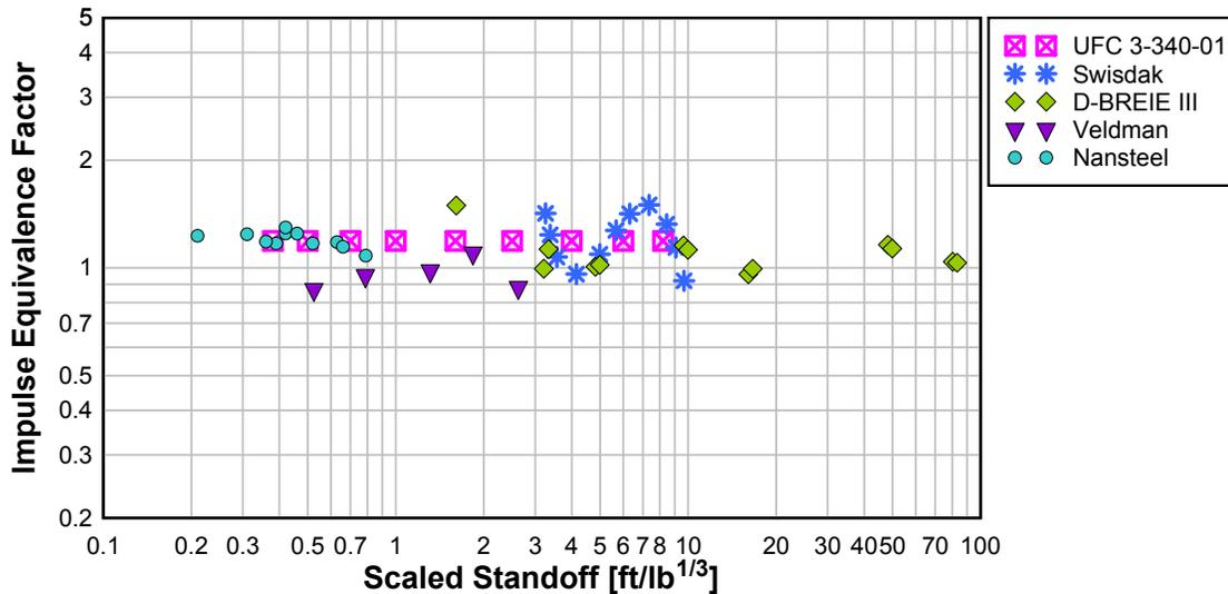
Figure 2: Impulse equivalence data for C-4 in STREET.
