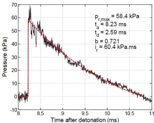
Figure 8: Typical curve fit used to determine peak pressure from gauge record (from [13]).
