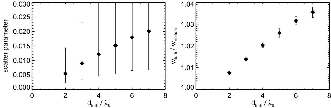
**Figure 6.** (Left) Median of the scattering parameter  $\alpha$  with the interquartile range as error bars and (right) average beam broadening as a function of the thickness of the turbulence region for the case of an average fluctuation level of  $\sigma \approx 4\%$  and an average structure size of  $L_c \approx 0.52 \lambda_0$ .
