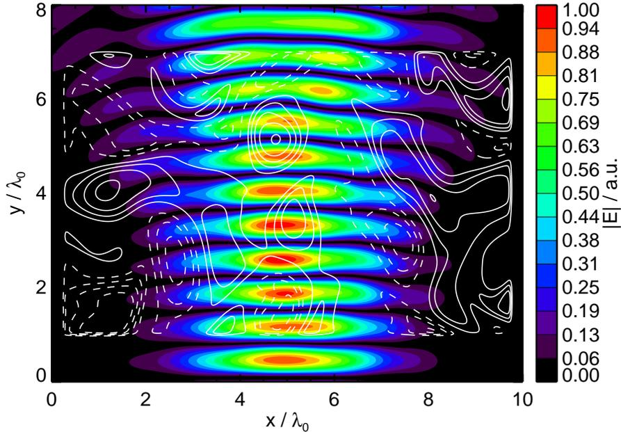
**Figure 5.** Contour plot of a snapshot of the absolute wave electric field together with the electron density fluctuations indicated by the white lines, where solid and dashed lines correspond to positive and negative perturbations (referring to the background electron density  $n_0$ ), respectively. Simulation parameters are  $L_c \approx 0.52 \lambda_0$ ,  $\sigma \approx 4\%$  and  $d_{\text{turb}} = 6 \lambda_0$ .
