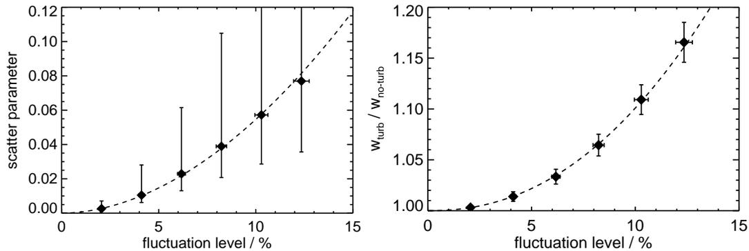
**Figure 7.** (*Left*) Median of the scattering parameter  $\alpha$  with the interquartile range as error bars and (*right*) average beam broadening as a function of the normalized fluctuation amplitude for the case of an average structure size of  $L_c \approx 0.52 \lambda_0$  and  $d_{\text{turb}} = 3 \lambda_0$ . The dashed line represents a power law fitted to the data.
