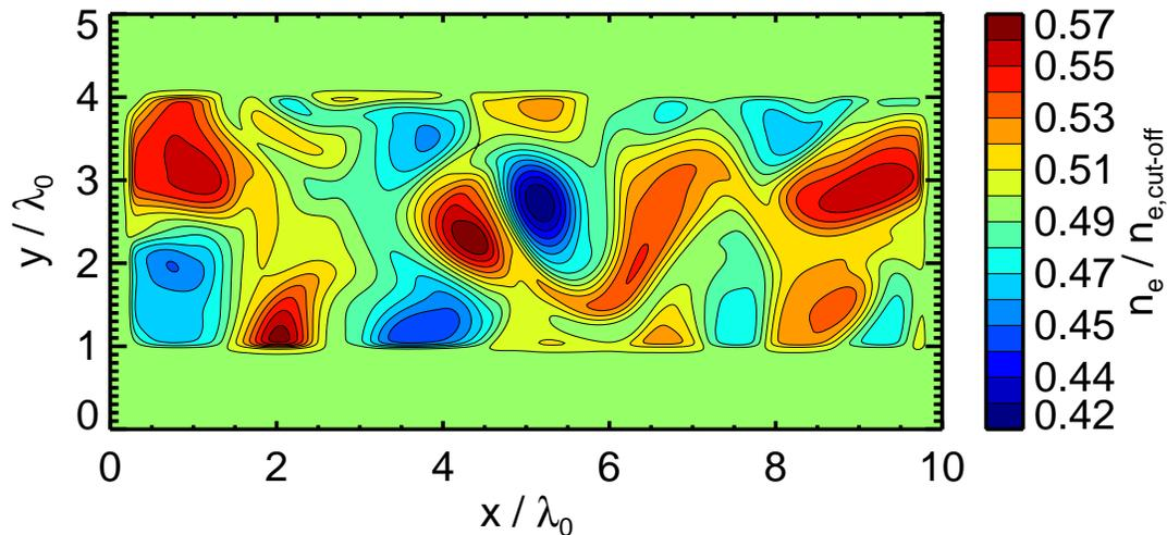
**Figure 1.** Contour plot of the electron density normalized to the O-mode cut-off density of the injected microwave for one of the grids which is used in the full-wave simulations. The microwave is injected from the bottom and detected at the top.
