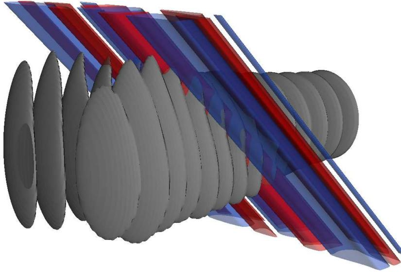
**Figure 9.** Snapshot of the positive wave electric field together with contours of the electron density fluctuations (red and blue corresponding to positive and negative perturbations respectively) for an angle of 45 degrees between the injected microwave beam and the electron density filaments.
