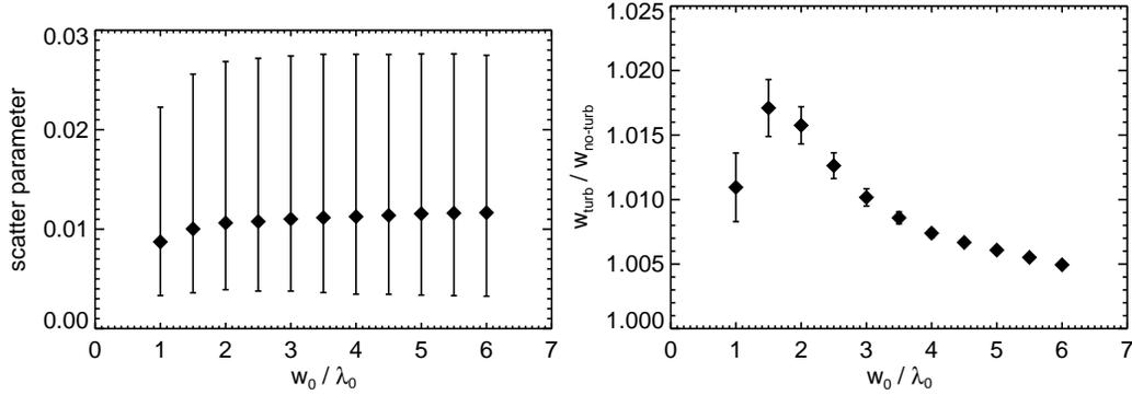
**Figure 8.** (Left) Median of the scattering parameter  $\alpha$  with the interquartile range as error bars and (right) average beam broadening as a function of the size of the beam waist for the case of an average fluctuation level of  $\sigma \approx 4\%$ , an average structure size of  $L_c \approx 0.52 \lambda_0$ , and a depth of the turbulence layer of  $d_{\text{turb}} = 3 \lambda_0$ .
