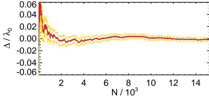
**Figure 3.** Average value of the spatial deviation of the maximum signal in the detector antenna plane as a function of the number of ensembles (the red central curve corresponds to the arithmetic mean and the upper and lower orange dashed curves correspond to the error given by the standard deviation of the mean).
