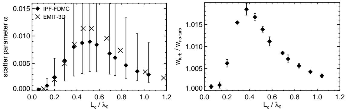
**Figure 4.** (Left) Median of the scattering parameter  $\alpha$  with the interquartile range as error bars and (right) average beam broadening as a function of the average structure size  $L_c$  for the case of an average fluctuation level of  $\sigma \approx 4\%$  and a size of the turbulence layer of  $d_{\text{turb}} = 3\lambda_0$ .
