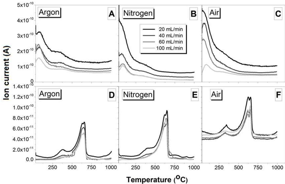
Fig 4. Mass spectroscopy results for  $\text{H}_2\text{O}_{(\text{g})}$  (A, B, C) and  $\text{CO}_2_{(\text{g})}$  (D, E, F) detected during TGA of an anhydrous GBFS, as a function of the gas environment
