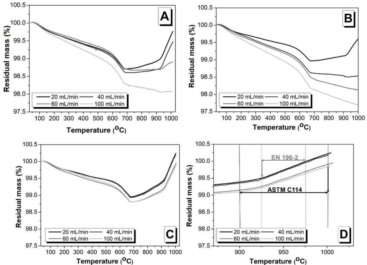
Fig 1. TGA results, as a function of the gas flowrate, of anhydrous GBFS tested under (A) argon, (B) nitrogen and (C) air at flowrates as marked, and (D) enlargement of the thermograms in air, highlighting ranges of temperatures used to determine LOI in EN and ASTM standards
