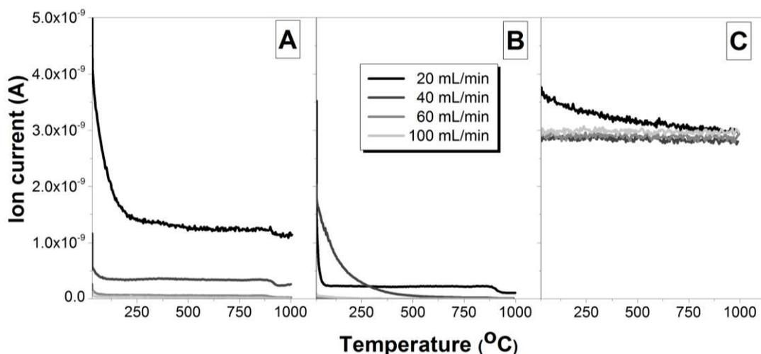
Fig 2. Mass spectra of O<sub>2(g)</sub> detected during TGA of an anhydrous GBFS when using (A) argon, (B) nitrogen or (C) air, as protective gases
