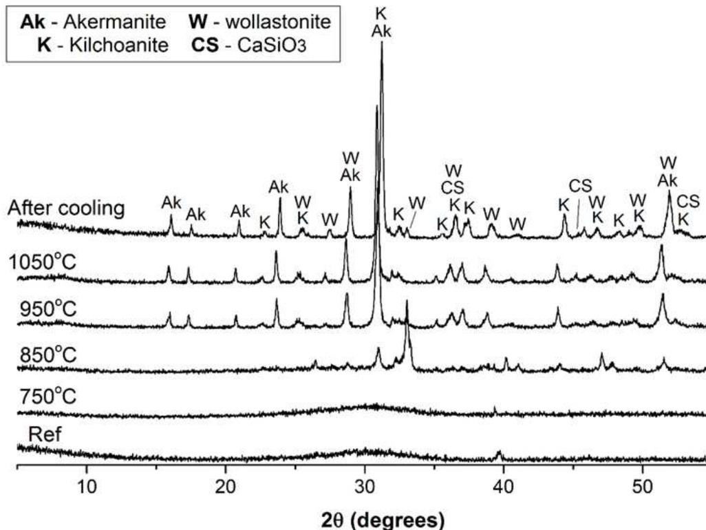
Fig 5. In-situ heating X-ray diffractograms (Cu K $\alpha$  radiation) of an anhydrous GBFS
