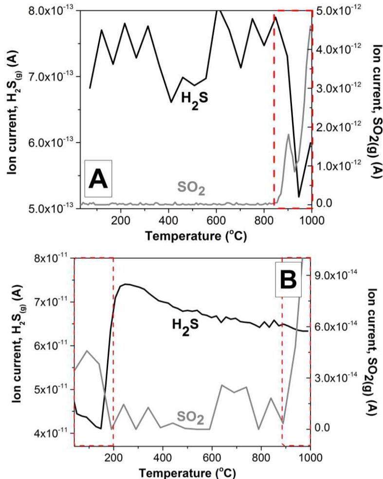
Fig 3. Mass spectroscopy results for H<sub>2</sub>S(g) and SO<sub>2</sub>(g) detected during TGA of anhydrous GBFS using 40mg of sample, and 20 mL/min of (A) N<sub>2</sub> or (B) air
