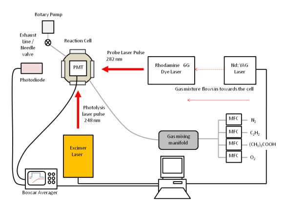
Figure S3. Schematic of the LFP/LIF system.
