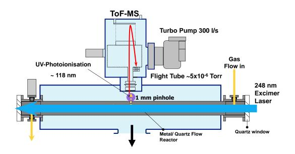
Figure S2. Details of the flow system, sampling and TOFMS.
