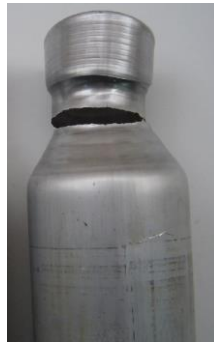
Fig. 34. Occurance of crack if nominal reduction of blank radius \Delta_i is too large [19].
