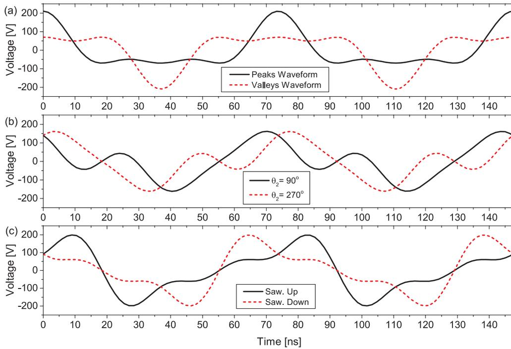
**Figure 2.** Examples of applied voltage waveforms over two consecutive RF periods for  $N = 3$  harmonics: (a) ‘Peaks’ (solid) and ‘Valleys’ (dashed) waveforms (equations (3) and (4)), (b) intermediate waveforms where  $\theta_2 = 90^\circ$  (solid) and  $\theta_2 = 270^\circ$  (dashed) and all other phases are zero (equations (3) and (4)), and (c) sawtooth up (solid) and down (dashed) waveforms (equations (3) and (5)).
