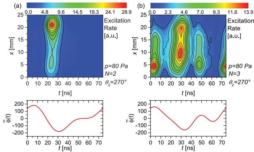
**Figure 11.** Spatio-temporal plots for  $\theta_2 = 270^\circ$  ( $\phi_{\text{tot}} = 210$  V) at 80 Pa of (a) the experimentally measured excitation rate for  $N = 2$  and (b) the experimentally measured excitation rate for  $N = 3$ . The applied voltage waveforms are shown below the spatio-temporal plots for reference.
