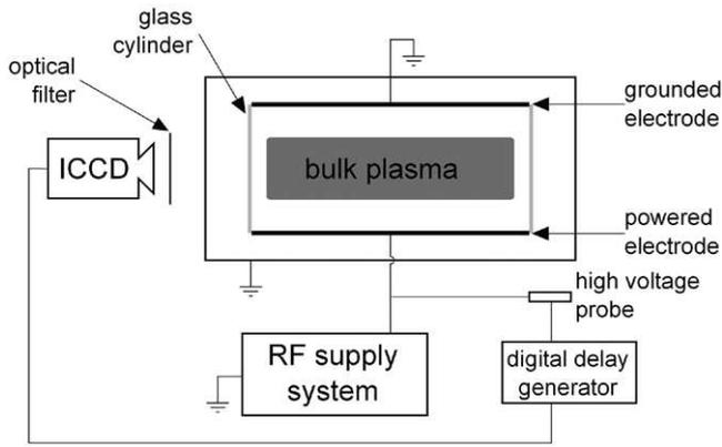
**Figure 1.** Sketch of the experimental setup consisting of a capacitively coupled GEC reference cell monitored by diagnostics (PROES via ICCD camera, and a high voltage probe for waveform monitoring/analysis).
