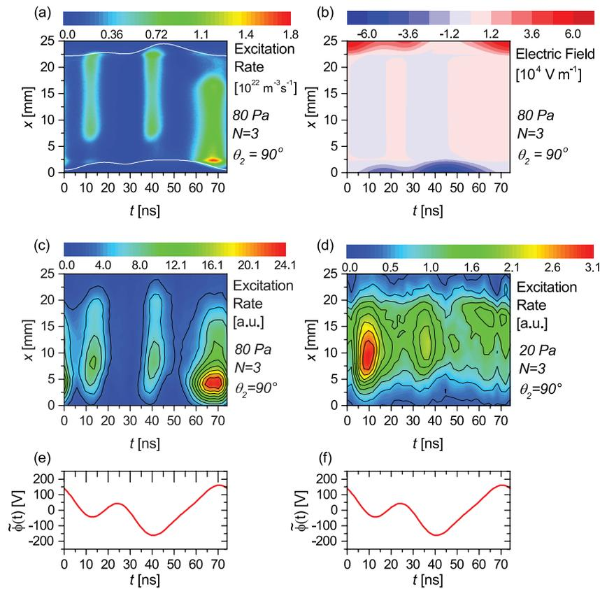
**Figure 10.** Spatio-temporal plots for  $\theta_2 = 90^\circ$  ( $N = 3$ ,  $\phi_{\text{tot}} = 210$  V) of (a) the excitation rate at 80 Pa obtained from the simulation with the sheath edges shown in white, (b) the electric field at 80 Pa obtained from the simulation, (c) the experimentally measured excitation rate at 80 Pa, and (d) the experimentally measured excitation rate at 20 Pa. The applied voltage waveform is shown in (e) and (f) for reference.
