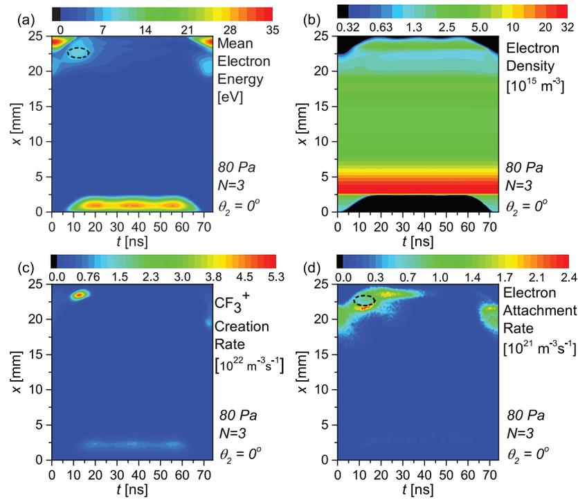
**Figure 8.** Spatio-temporal plots for 80 Pa,  $\theta_2 = 0^\circ$  ('Peaks' waveform,  $N = 3$ ,  $\phi_{\text{tot}} = 210$  V) of (a) mean electron energy, (b) electron density, (c) rate of  $\text{CF}_3^+$  creation, and (d) rate of electron attachment (i.e.  $\text{CF}_3^-$  and  $\text{F}^-$  creation), as obtained from the simulation.
