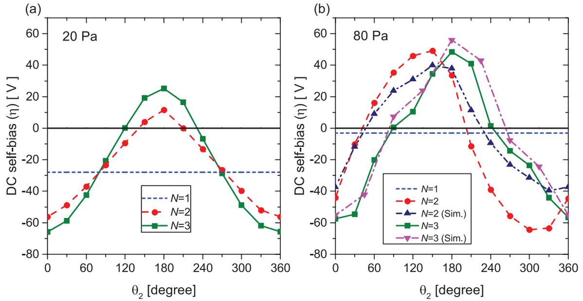
**Figure 5.** DC self-bias as a function of  $\theta_2$  for (a) 20 Pa (experimentally measured bias) and (b) 80 Pa (including both the experimentally measured bias and the bias obtained from the PIC simulation, a.k.a. ‘Sim.’) for different numbers of applied harmonics,  $N = 1, 2, 3$ .  $\phi_{\text{tot}} = 210$  V for all cases.
