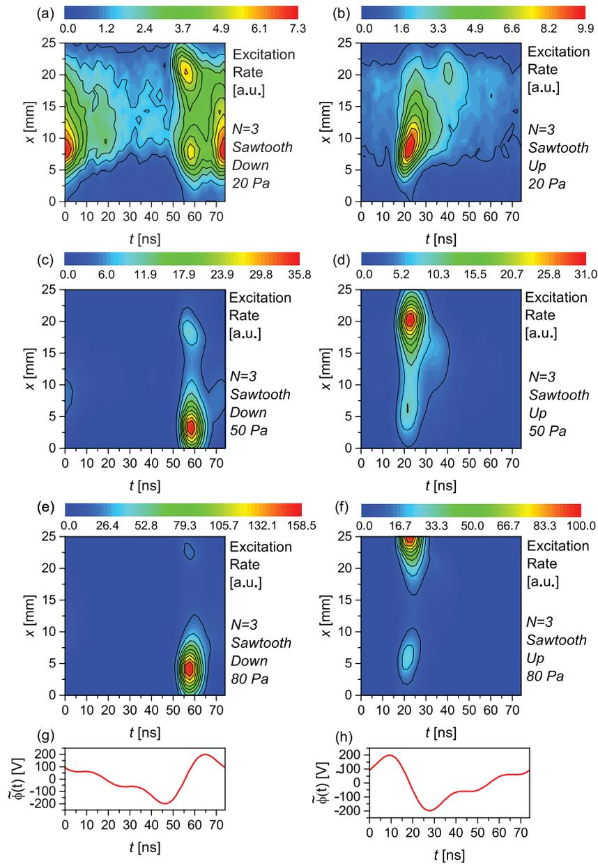
**Figure 13.** Experimentally measured spatio-temporal excitation rate for sawtooth waveforms ( $N = 3, \phi_{\text{tot}} = 253$  V) at ((a)–(b)) 20 Pa, ((c)–(d)) 50 Pa, and ((e)–(f)) 80 Pa. The left column contains the sawtooth down ( $\theta_2 = 90^\circ, \theta_3 = 180^\circ$ ) results, while the right column shows the sawtooth up ( $\theta_2 = 270^\circ, \theta_3 = 180^\circ$ ) results. The applied voltage waveforms are shown in (g) and (h) for reference.
