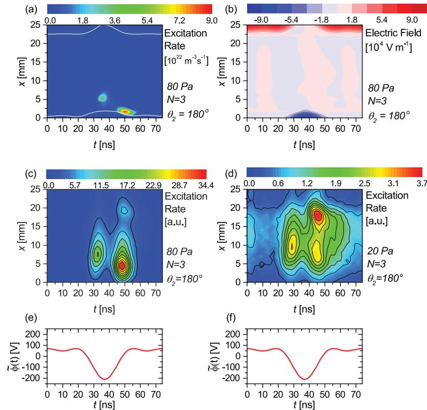
**Figure 9.** Spatio-temporal plots for  $\theta_2 = 180^\circ$  ('Valleys' waveform,  $N = 3$ ,  $\phi_{\text{tot}} = 210$  V) of (a) the excitation rate at 80 Pa obtained from the simulation with the sheath edges shown in white, (b) the electric field at 80 Pa obtained from the simulation, (c) the experimentally measured excitation rate at 80 Pa, and (d) the experimentally measured excitation rate at 20 Pa. The applied voltage waveform is shown in (e) and (f) for reference.
