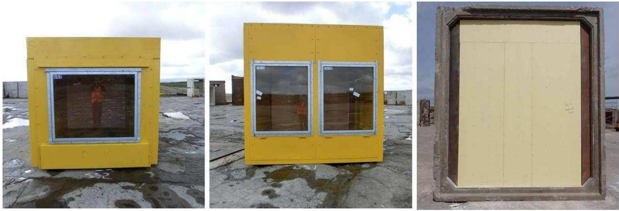
Figure 1 – Typical glazing targets mounted in a single aperture cubicle and a double aperture cubicle, and a typical wall target mounted in a reinforced concrete cubicle
