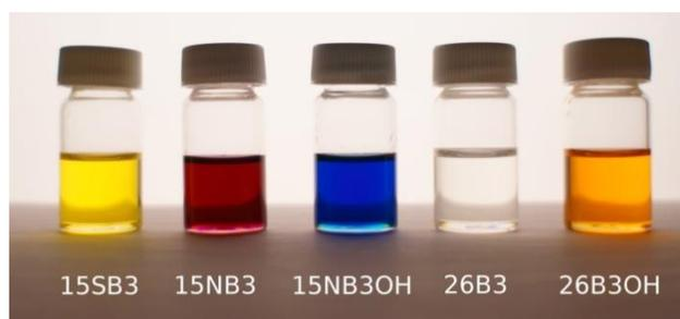
**Figure 3.** A photograph of solutions of the dyes at ca.  $2 \times 10^{-4} \text{ mol dm}^{-3}$  in *p*-xylene.
