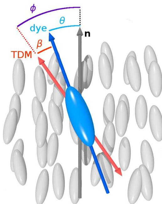
**Figure 1.** Schematic representation of a dye molecule (blue) within a nematic liquid crystal host (grey). The average orientation of the host molecules is given by the director,  $\mathbf{n}$ , and the relative orientations of the long molecular axis of the dye (blue) and the TDM of the dye (red) are given with angles defined.
