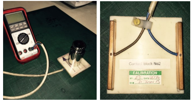
Fig. 3. The sheet conductance test setup (left) and the measurement electrodes (right).
