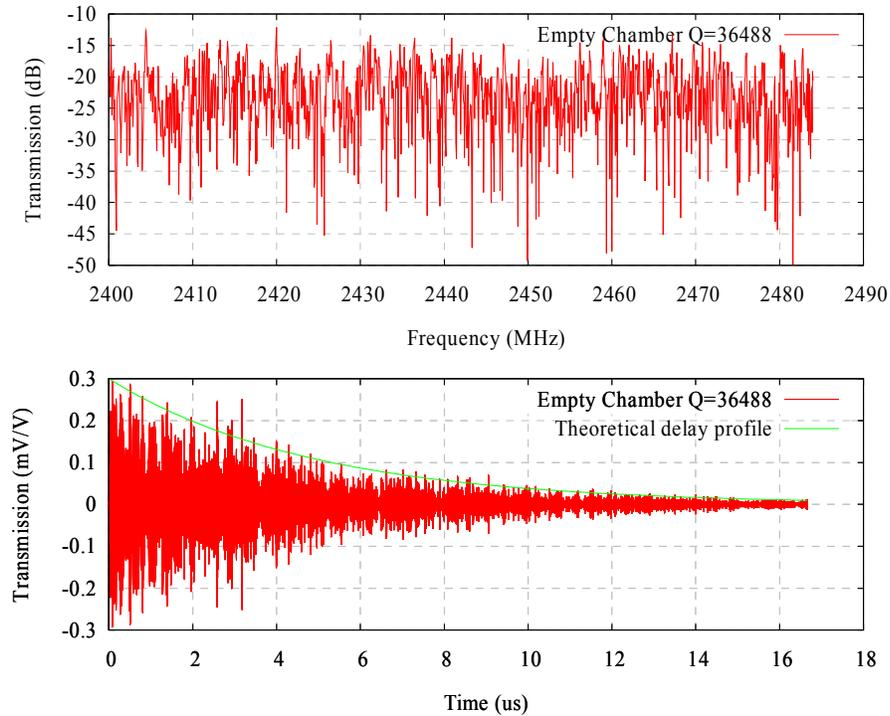
Figure 3: Time and frequency response for transmission ( $S_{21}$ ) between two ZigBee quarter wave antennas in the large reverberation chamber from 2.4GHz to 2.484GHz for the empty chamber (no absorber)
