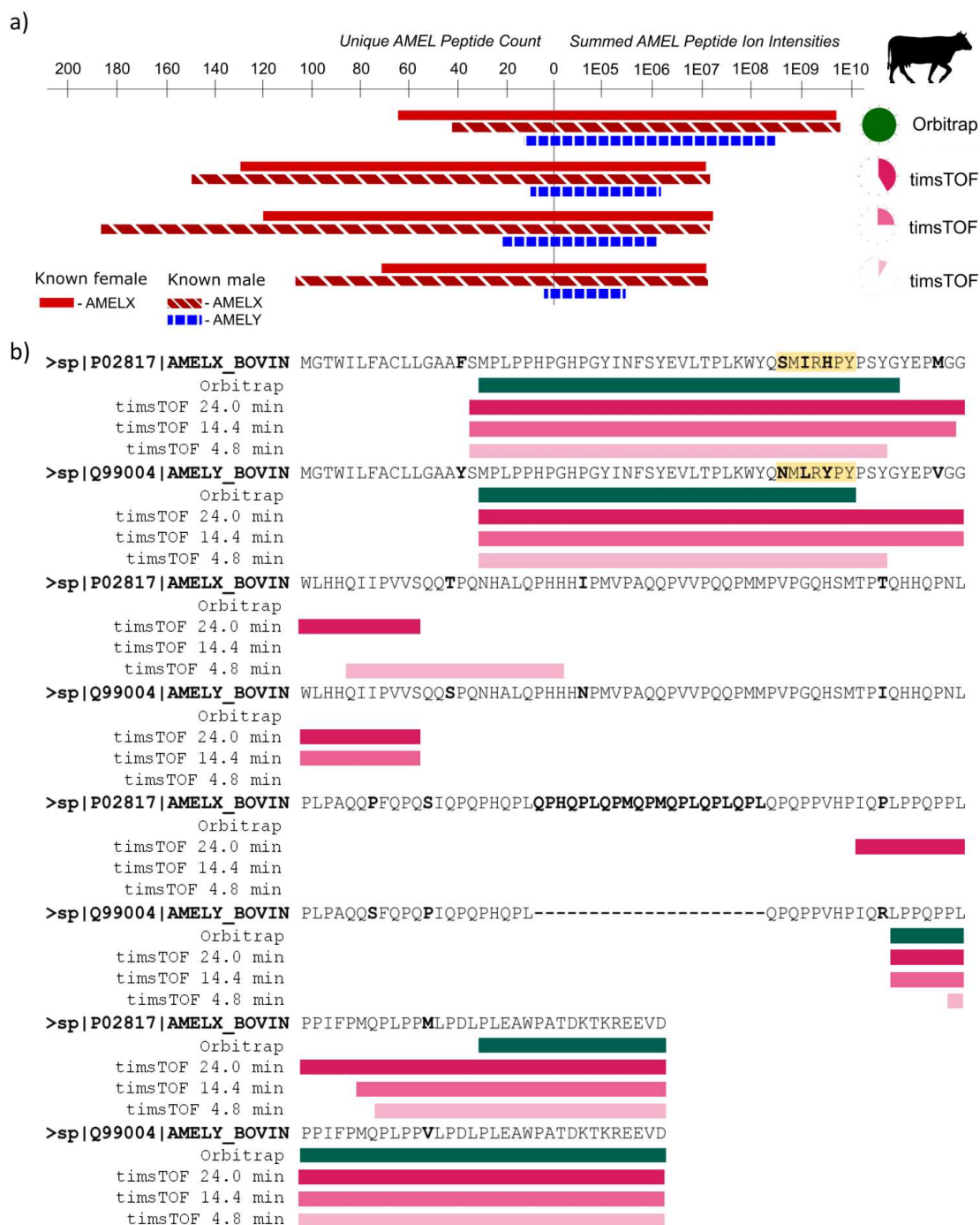
Figure 4. a) Unique AMELX (red) and AMELY (blue) peptide counts (left) and summed AMELX (red) and AMELY (blue) peptide ion intensities (right) from powdered enamel from a modern female (filled bars) and male (hashed bars) Bos taurus tooth when analysed by Orbitrap Fusion MS, and three different Evosep-timsTOF MS methods (24.0 minute, 14.4 minute, and 4.8 minute). b) Aligned bovine AMELX (Uniprot accession number P02817) and AMELY (Uniprot accession number Q99004) protein sequences, showing the protein coverage observed in the modern male tooth across the different MS methods. Bold letters indicate where there are differences in the AMELX and AMELY sequence. The yellow highlighted regions indicate the regions where most dimorphic peptides are identified in bovine samples.
