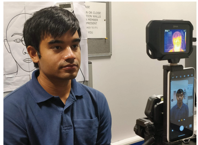
Fig 1. The FLIR C3 IR camera workstation with participant alignment, digital photography and IR thermography. IR = infrared.
