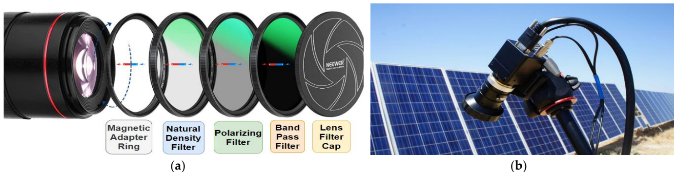
Figure 2. Optical filter design architecture for the EL camera: (a) Layers of the EL camera layout; (b) Physical EL camera next to PV installation.
