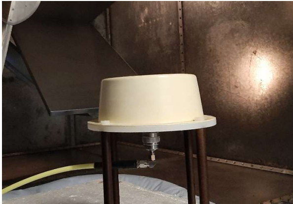
Fig. 4. Biconical dipole antenna EUT in the reverberation chamber
