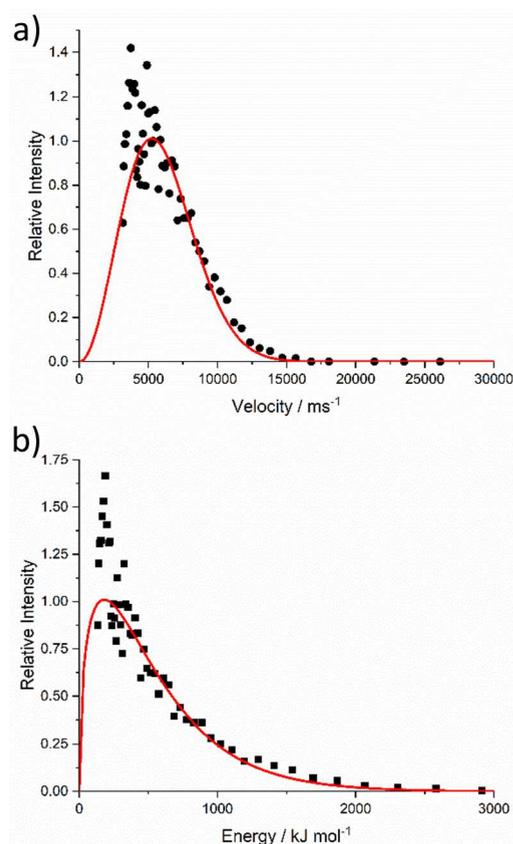
**Figure 5.** (a) Speed distribution and (b) kinetic energy distribution of the Al atoms derived from the appearance profiles in Figure 4. Red lines are best-fit Maxwell–Boltzmann distributions over the ranges of speed or energy, corresponding to the first 150  $\mu$ s of the appearance profile. The experimental data are peak-normalized to the fits. Data at slower speeds/lower energies have been binned and averaged to improve visual clarity.
