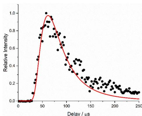
**Figure 4.** Al atom appearance profiles recorded on the  $^2D_{5/2} \leftarrow ^2P_{3/2}^o$  (226.910 nm) transition, produced with an ablation energy of 8 mJ pulse $^{-1}$ . Time zero corresponds to the ablation laser pulse. No target surface was present. The best-fit Maxwell–Boltzmann distribution to the first 150  $\mu$ s is shown in red.
