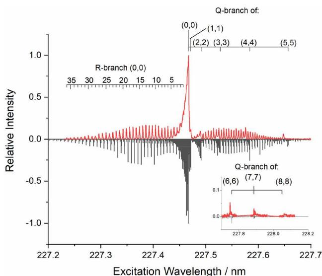
**Figure 7.** AIF excitation spectrum obtained from the reaction of Al with a liquid PFPE sample in our initial test system (upper trace) and PGOPHER simulation (lower trace) using a rotational temperature of 300 K and a synthesis of several vibrational temperatures up to 1500 K.
