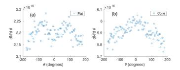
FIG. 12. (a), (b) Electron angular distribution for flat Al (left) and cone Al (right).
