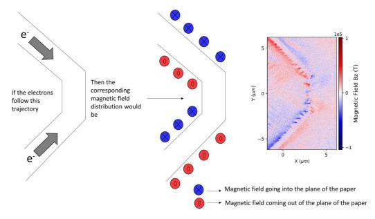
FIG. 11. Tracing of charged particles with directionality of magnetic fields at t = 0.15 ps.
