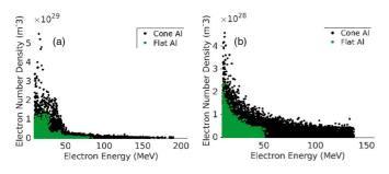
FIG. 9. (a), (b) Electron number density corresponding to their energy at the end of the laser pulse (left) and at the end of the simulation (right). Each dot represents an individual grid cell with the x coordinate being the electron energy associated with it and its corresponding electron density denoted by the y coordinate.
