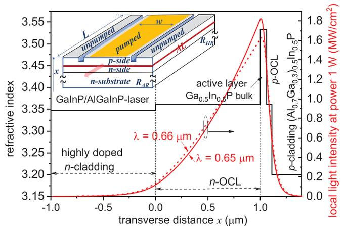
**Figure 1.** Schematic of the refractive index profile of the laser structure and the waveguide mode intensity distribution for the wavelength of 650 nm (solid), 660 nm (dashed). The inset shows a typical 3D structure possible, with the  $n$ -side comprising the  $n$ -cladding and the  $n$ -OCL and the  $p$ -side, the  $p$ -cladding and the  $p$ -OCL. Active stripe width  $w = 100 \mu\text{m}$ .
