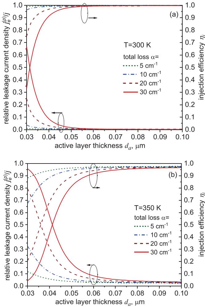
**Figure 6.** The ratio of the leakage to total current and the injection efficiency as functions of the active layer thickness for different values of the total cavity loss and the temperature 300 K (a) and 350 K (b).
