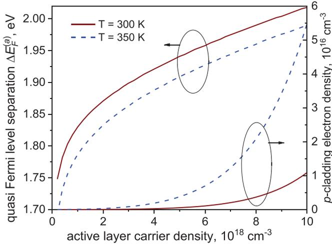
**Figure 4.** The electron and hole quasi Fermi level separation and the corresponding density of electrons thermally excited in the  $p$ -cladding for the designs of figures 1, 2 and different temperature values as function of active layer carrier density.
