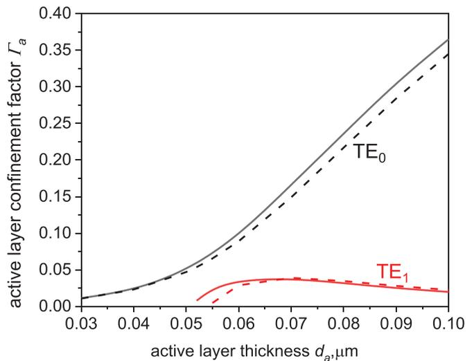
**Figure 2.** Confinement factors of the optical modes as function of the active layer thickness for the structure of figure 1: solid line:  $\lambda = 650 \text{ nm}$ ; dashed line— $\lambda = 660 \text{ nm}$ .
