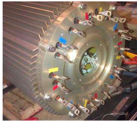
Figure 1. A fin-cooled electric tail motor [19].
