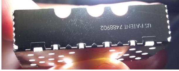
Fig. 13. Shield 1 with back illuminations showing gaps.
