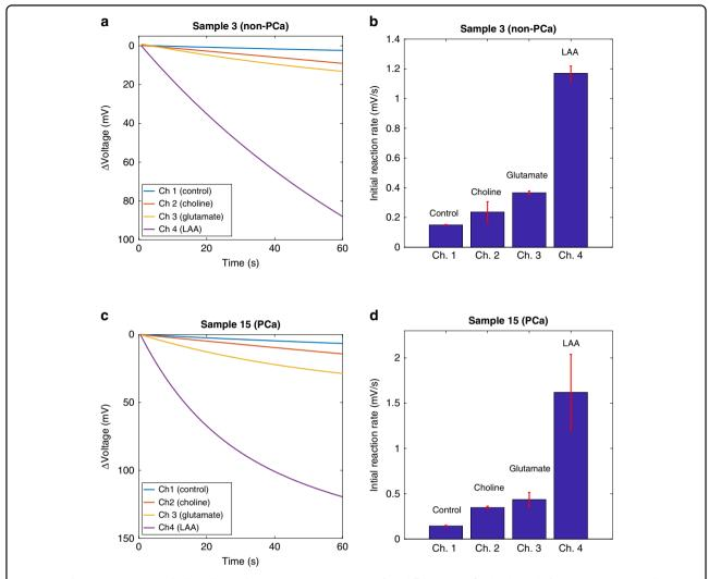
**Fig. 7 Simultaneous testing with clinical samples. a** Initial reaction rates in four different microfluidic channels for a non-PCa sample. **b** Output from different microchannels for a non-PCa sample. **c** Initial reaction rates in four different microfluidic channels for a PCa sample. **d** Output from different microchannels for a PCa sample.
