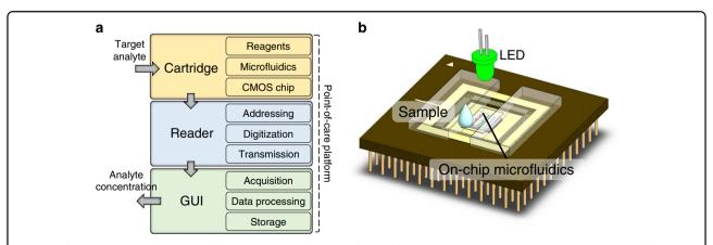
**Fig. 1 Platform architecture and cartridge. a** Schematic architecture of the platform showing the cartridge that needs only a drop of sample to perform a measurement, the reader, and the computing device for use as a GUI. **b** A sketch of the multiple measurement cartridge device used in this work with a CMOS chip, passive microfluidics, a chip package, and an optical assembly.
