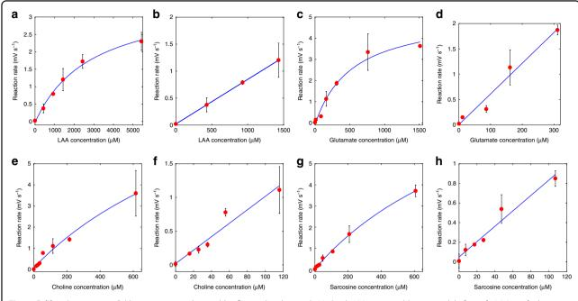
Fig. 3 Calibration curves. Calibration curves obtained by fitting the data with Michaelis–Menten and linear models for **a**, **b** LAA, **c**, **d** glutamate, **e**, **f** choline, and **g**, **h** sarcosine in human plasma.
