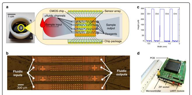
**Fig. 2 Cartridge and reader. a** The cartridge (left) and schematic diagram of its main components (right). **b** Micrograph of the microfluidics fabricated on the chip's sensitive area. **c** Profile of the microstructure built on the sensitive area measured with a Bruker Contour GT-X 3D Optical Profiler (**d**). The handheld reader removed from its enclosure.
