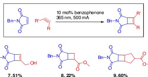
**Scheme 3.** Intermolecular [2+2]-cycloaddition general reaction scheme and scope.
