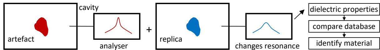
Figure 1. Principle of Dielectric Replica Measurement (DRM)
