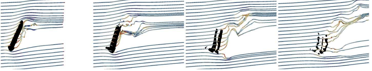
Figure 9. Streamlines in simulation m10c2l8o30 at t = 0.88, 1.58, 2.28 and 2.98 t_{cs} . The streamlines are in the Y = 0 plane and are introduced at X = -5 . They are colour coded with the velocity from dark red (low speed) to dark blue (high speed). The black surface is a contour at the original filament density.
