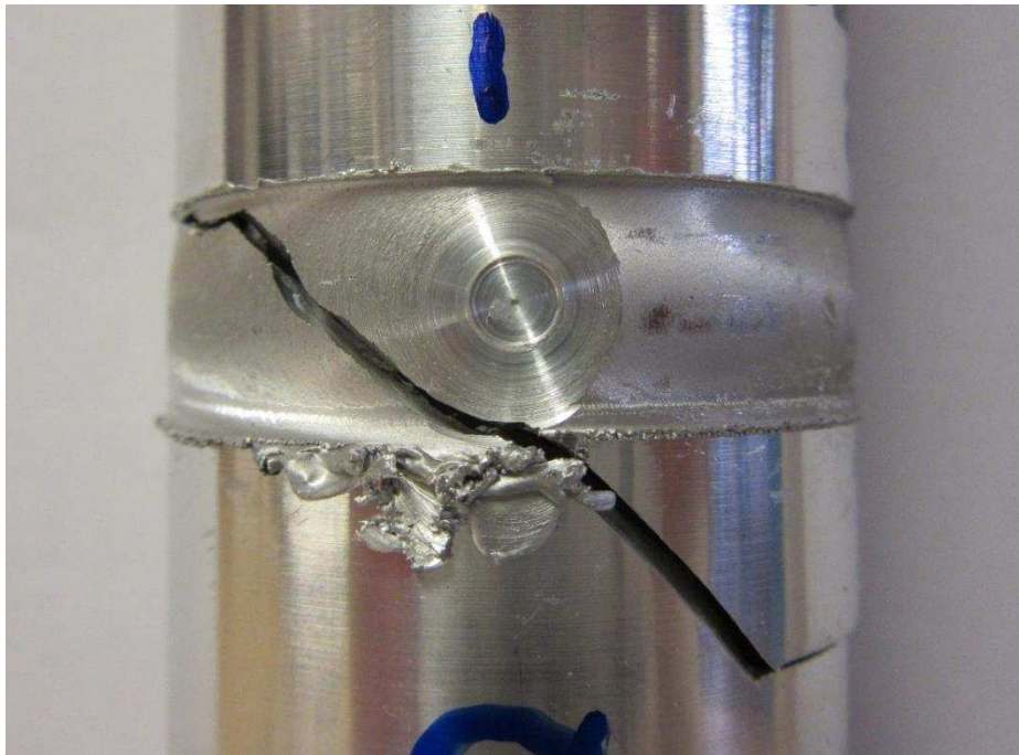
Figure 12 Certain tension-torsion specimens showed crack initiation associated with the stop-start position. This is specimen IPh8.
