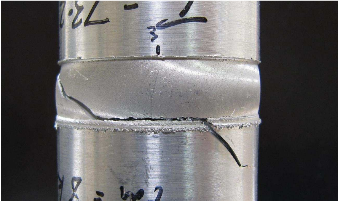
Figure 9 In-phase tension-torsion fatigue test (IPh21) showing that the crack has initiated along the tool shoulder groove on the retreating side and then moved across to the advancing side of the weld.
