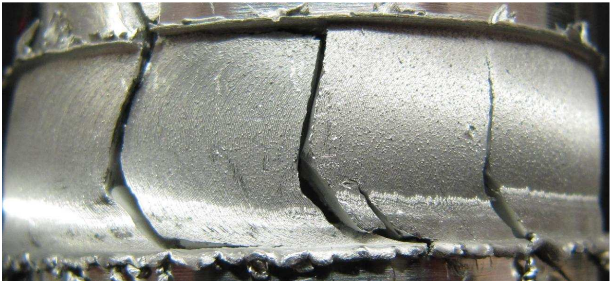
Figure 11 Multiple crack initiation appears to be exacerbated at lower torsional stress and hence longer fatigue lives. This image shows specimen T16.
