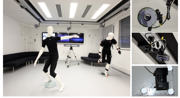
Figure 3. The BTS SMART-D system used for this study and the BSN node mounted with reflective markers for orientation accuracy evaluation.
