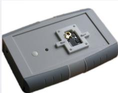
Figure 2. Current solution of reading in the EEG data, a docking station.
