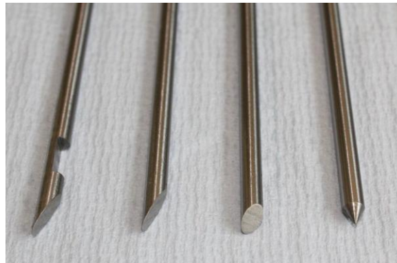
Fig. 2 Scale models of the types of needle tip: (a) Westcott, (b) Chiba (25° bevel), (c) Turner (45° bevel) and (d) 60° Cone.
