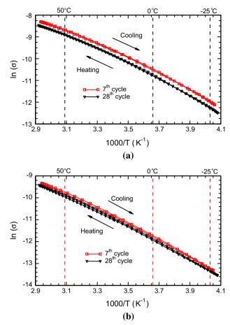
Fig. 6 Arrhenius plots for a GGBS/35 concrete (w/b = 0.65), and, b FA/35 concrete (w/b = 0.35) at 7th and 28th cooling/heating cycle presented over the temperature range +70/-30 °C
