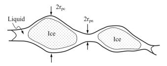
**Fig. 4** Schematic representation of 'ink-well' model for capillary pore structure showing pore cavities (of diameter  $2r_{pc}$ ) connected through pore necks (of diameter  $2r_{pn}$ )
