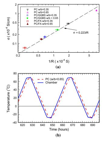
Fig. 2 a Calibration curve for embedded electrodes, and, b temperature of environmental chamber and internal temperature of specimen
