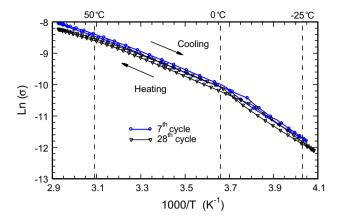
Fig. 7 Arrhenius plots for GGBS/35 concrete (w/b = 0.65) at 7th and 28th cooling/heating cycle over the temperature range +70/-30 °C
