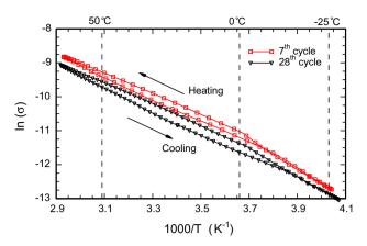
Fig. 8 Arrhenius plots for FA/35 concrete (w/b = 0.65) at 7th and 28th cooling/heating cycle presented over the temperature range +70/-30 °C
