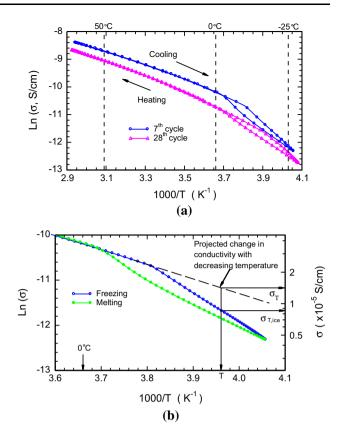
Fig. 3 Arrhenius plots for **a** PC concrete (w/b = 0.35) at 7th and 28th cooling/heating cycle presented over the temperature range +70/-30 °C; **b** close-up of low-temperature end of Arrhenius plot during 7th cycle
