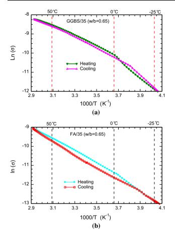
Fig. 9 Showing hysteresis in the Arrhenius plot (28th cycle) over the temperature range +70/-30 °C for a GGBS/35 concrete, and, b FA/ 35 concrete (both w/b = 0.65)
