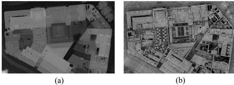
Figure 12: Comparison between roof detail visualisation in an elevation image (a) and an occlusion image (b). Pixel dimensions are \Delta x = \Delta y = 0.25 \text{ m} in both images. Note that neither of these images were contrast enhanced after being cropped out of larger images.
