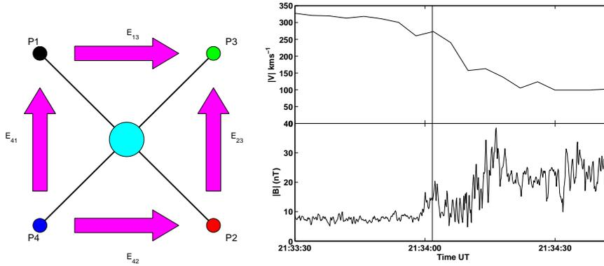
**Fig. 24** The left panel shows the configuration of the EFW electric field probes and illustrates the electric fields calculated from them. The right hand panel shows the magnitude of the magnetic field (bottom) and ion bulk flow (top) measured during the shock crossing that occurred on February 26<sup>th</sup>, 2002 at 2134 UT. (Adapted from Balikhin et al. 2005).
