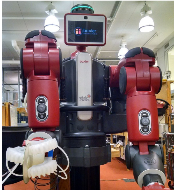
Fig. 1: The soft robotic hand, mounted to the wrist of a Baxter robot, is picking up a sample object.
