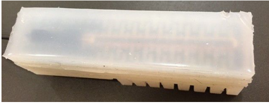
Fig. 4: This is a view of the inside of the finger. Through the translucent rubber, the constraint layer and the bend sensor are visible.
