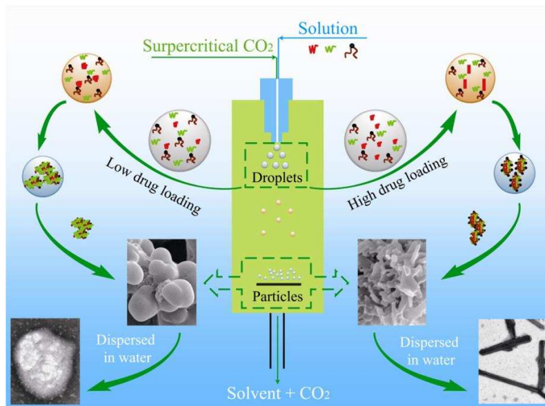
Fig. 13. Schematic representation of obtained spherical or clavate HCPT-PL under different drug loading.
