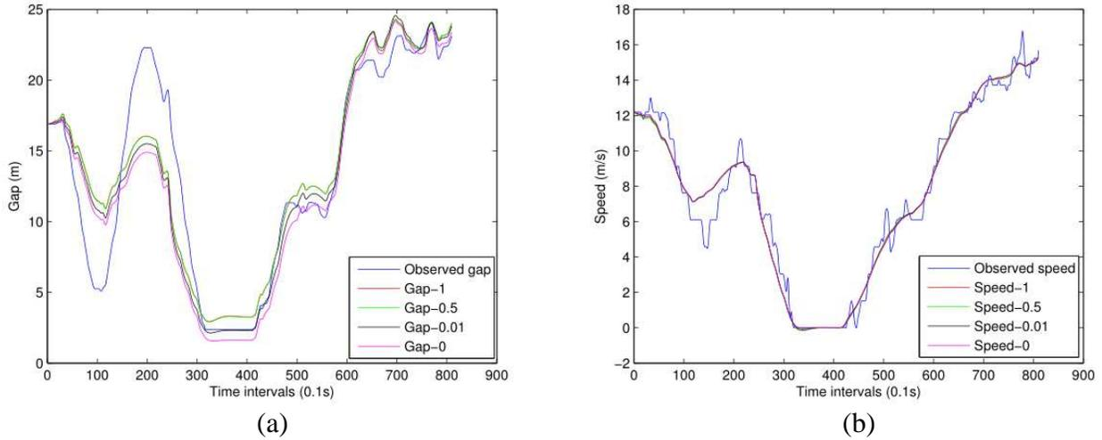
**FIGURE 1 Comparison of three calibrated and observed data for (a) gap and (b) speed ('Gap-1' means the case of  $\lambda = 1$ ).**
