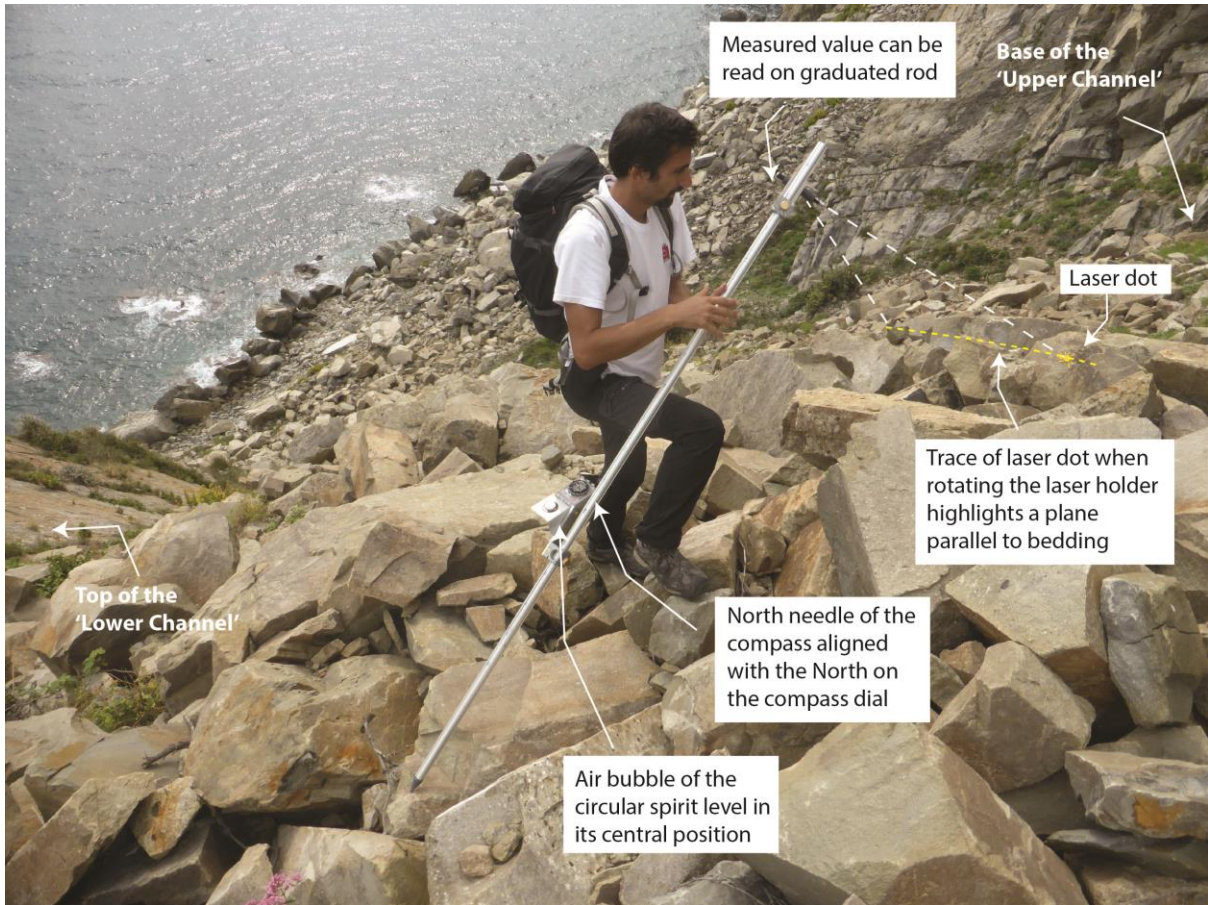
269 Figure 3. The new Jacob's staff in action, measuring the stratigraphic thickness of the covered 270 interval between the top of the 'Lower Channel' and the base of the 'Upper Channel' at the 271 Monterosso outcrop (Gottero Sandstones, NW Italy). Photo courtesy of Marco Fonesu.
