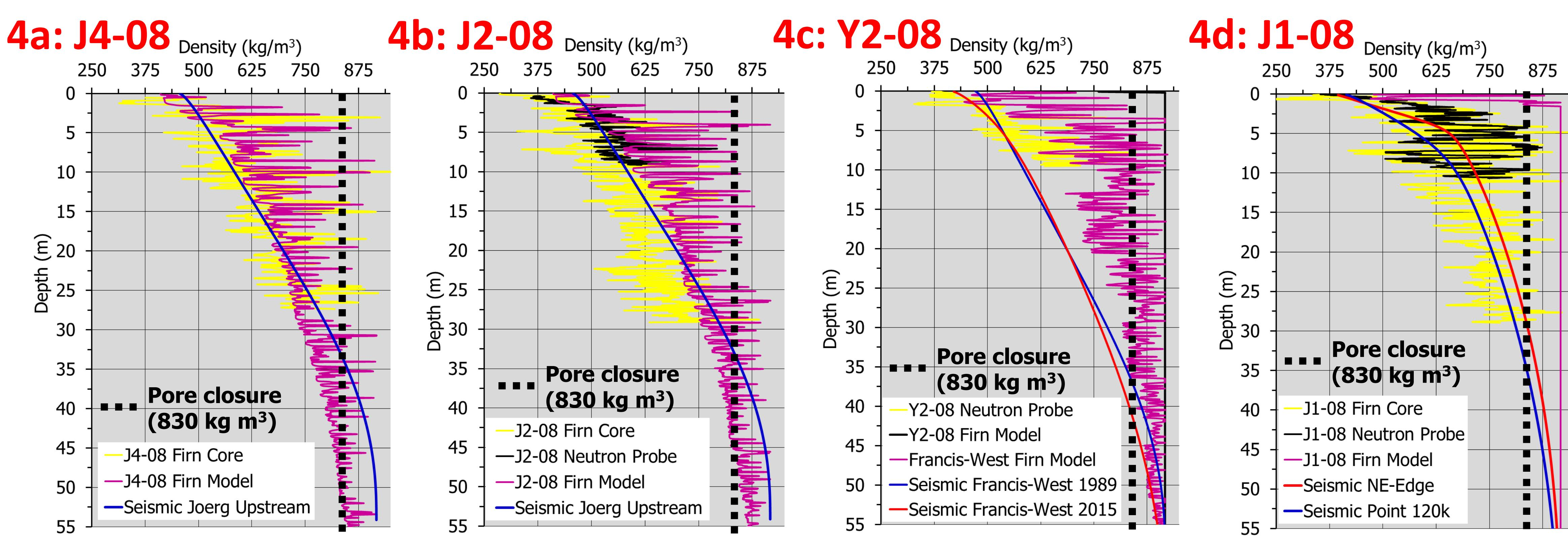
Comparison of depth-density profiles from seismic and borehole (gravimetric firn core analysis, neutron probe) data (note that seismic and borehole acquisitions are not precisely co-located), with simulations from the 1-D firn model.
