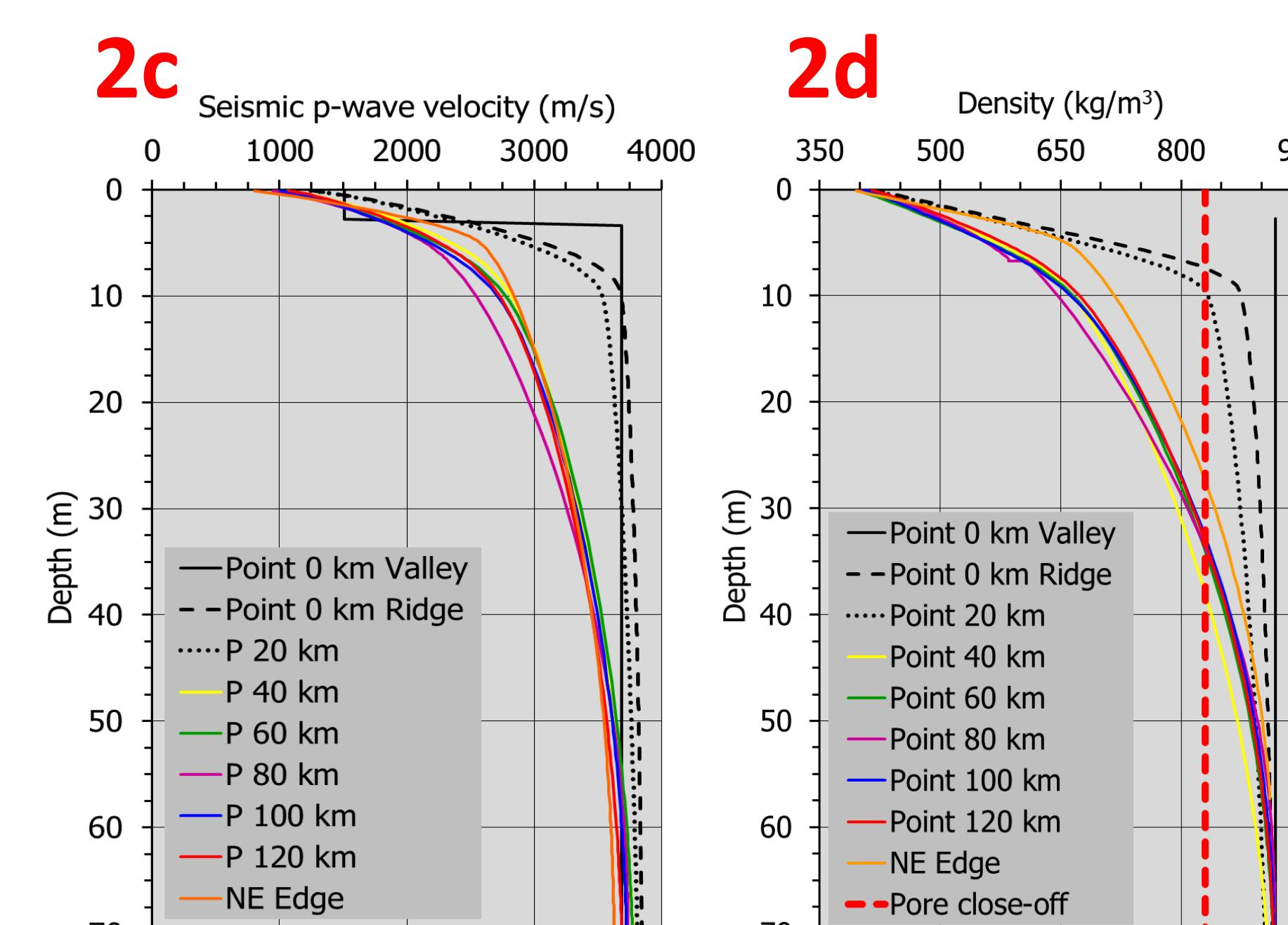
Depth profiles of p-wave velocity and density along transect from Point 0k to NE-Edge
