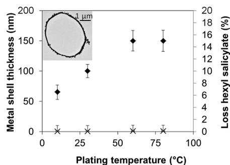
**Figure 6.** (◆) Thickness of metal shell as a function of plating temperature, measured from microtome images using TEM, and (×) release of core as a function of plating temperature (4:1 ethanol–water mixture for 7 days at 40 °C). (Inset) TEM image showing a microtomed capsule from which shell thicknesses are measured. A high-magnification image of part of this cross section is shown in the Supporting Information.
