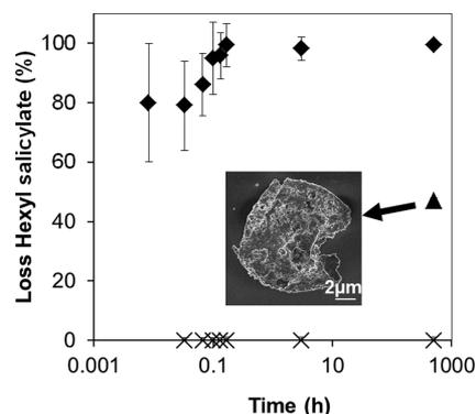
**Figure 5.** (◆) Hexyl salicylate release profile from PMMA capsules and (×) gold coated PMMA capsules, placed in 4:1 ethanol–water at 40 °C. (▲) Release of encapsulated oil observed from mechanically fractured gold coated capsules (after residing in ethanol–water mixture for 7 days). (Inset) SEM image of a mechanically fractured gold coated PMMA capsule with hexyl salicylate core.
