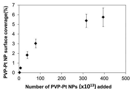
**Figure 4.** TEM data showing how the concentration of PVP-Pt NPs in the continuous phase affects the resulting adsorption density of the NPs on the polymeric microcapsule surface (conversion of number NPs per  $\mu\text{m}^2$  to percentage surface coverage used mean diameter of NPs).
