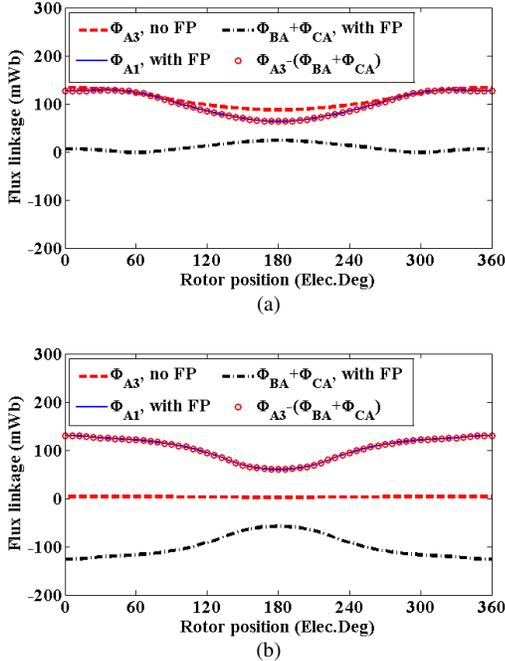
Fig. 5 Flux linkage separation for CSRSM and MCSRM supplied by 3-phase dc current using FP method. Phase current is 40A to make sure both machines are heavily saturated. (a) CSRSM, (b) MCSRM.  $\Phi_{A1}$  stands for the self flux of phase A, while  $\Phi_{A3}$  stands for total flux of phase A (self + mutual fluxes).
