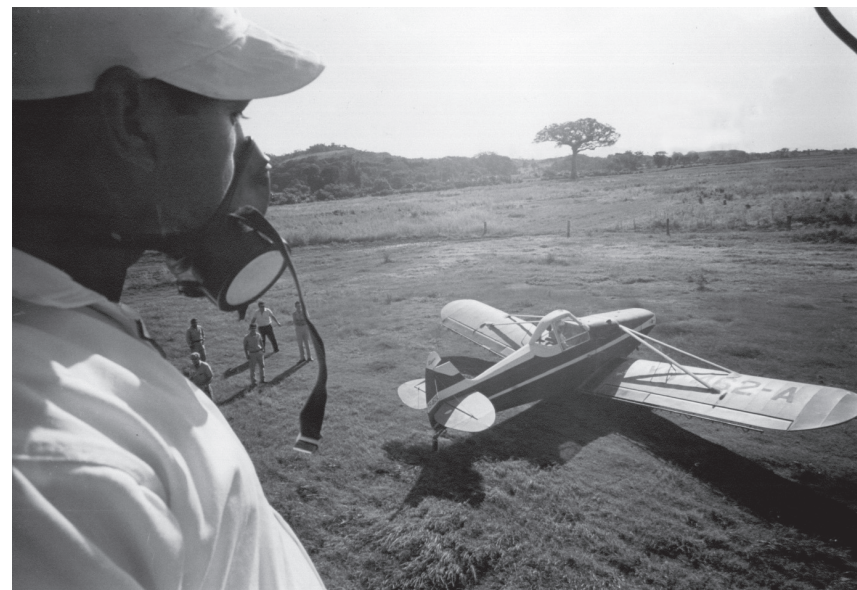
El Salvador, 1960s. Piper PAWNEE crop-dusting plane, loaded with 90 gallons (US) of dilute water emulsion of the organophosphorus insecticide, fenthion to be used as an anopheline larvicide on the breeding places of Anopheles albimanus nearby. WHO/Utaka Nagarta
