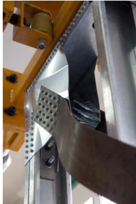
Figure 8. (a) Net section failure for WLE-C2 and (b) brace yielding for WHD-C2
