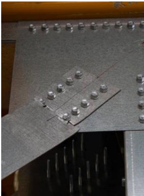
Figure 8. (a) Net section failure for WLE-C2 and (b) brace yielding for WHD-C2
